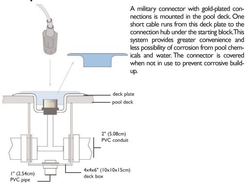
\*The Quick Connect Deck Plate system (or an on-deck cable harness) is required to accommodate speedlights on the front of RJPs.
